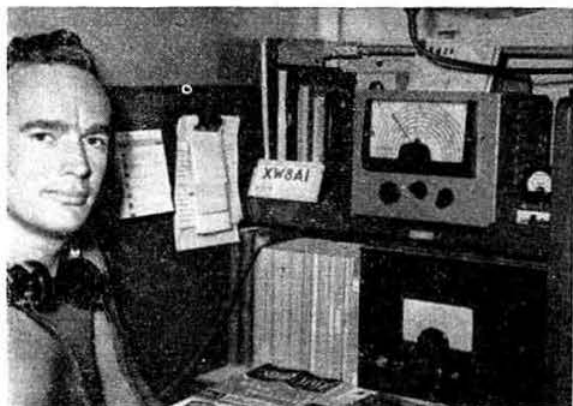
G3JFF/M on board H.M.S. Cook from January 1961 to September 1962. The transmitter was a Panda Cub while a Geloso front end feeding a B40 was used for reception. The aerial was a 15m vertical.
